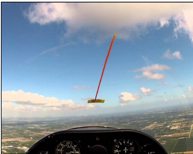
Figure 18-7. A string attached to the windshield of gyroplane is often used to indicate rotation about the yaw axis. An inclinometer may also be used.
