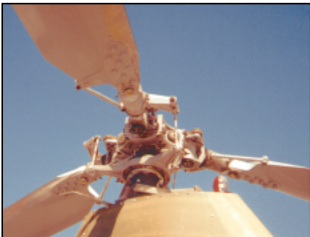
Figure 18-2. The fully articulated rotor system enables the pilot to effect changes in pitch to the rotor blades, which is necessary for jump takeoff capability.
