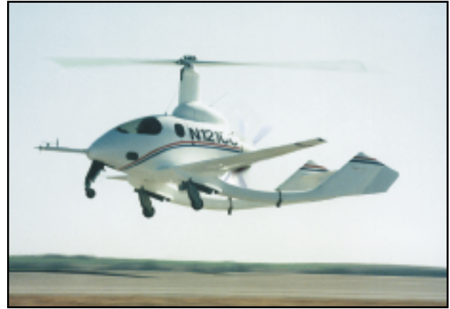
Figure 15-3. The CarterCopter uses wings to enhance performance.
