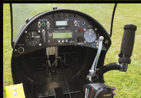
Plans and parts for this single-seat ultralight are produced in Florida. It is powered by a 65-hp Rotax 582 with a three-blade Warp drive propeller. It features 24-foot Dragon Wing rotor blades with a hydraulic pre-rotator, light-weight basic instruments, and rotor tachometer. Centerline thrust and a tall tail help stabilization in all power settings.
