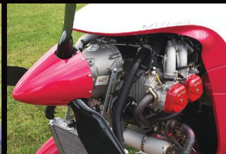
Produced in Germany, the 2017 MTOSport includes heated seats with lumbar support. It’s powered by a turbocharged 115-hp Rotax 914 engine. The panel features a Garmin 796 GPS and electronic airspeed indicator, Funke comm radio, and Mode S transponder. It also has a pneumatic clutch pre-rotator.
