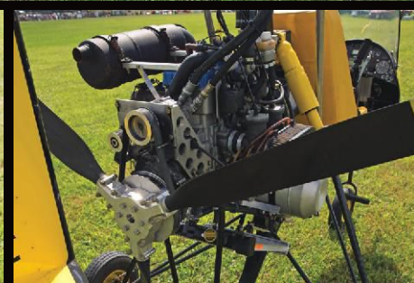
Plans and parts for this single-seat ultralight are produced in Florida. It is powered by a 65-hp Rotax 582 with a three-blade Warp drive propeller. It features 24-foot Dragon Wing rotor blades with a hydraulic pre-rotator, light-weight basic instruments, and rotor tachometer. Centerline thrust and a tall tail help stabilization in all power settings.
