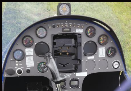
Produced in Germany, the 2017 MTOSport includes heated seats with lumbar support. It’s powered by a turbocharged 115-hp Rotax 914 engine. The panel features a Garmin 796 GPS and electronic airspeed indicator, Funke comm radio, and Mode S transponder. It also has a pneumatic clutch pre-rotator.
